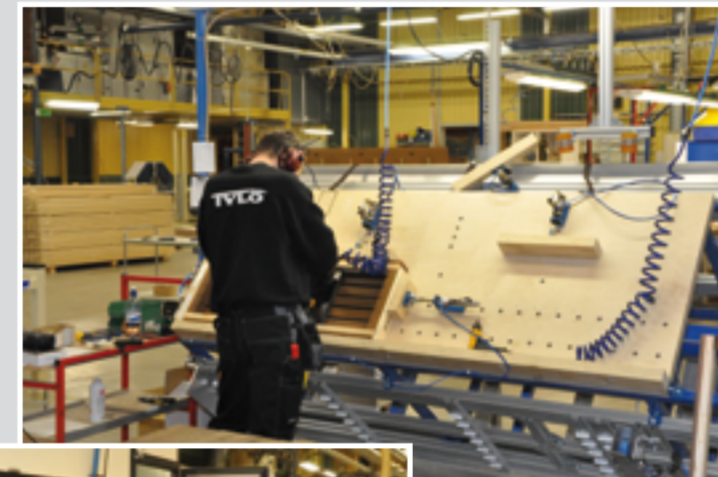
Manufacture of a sauna bench
